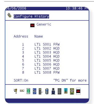
Having selected 'Generic' the available connected controllers will be displayed. The list will indicate the controllers net ID address and the description.
