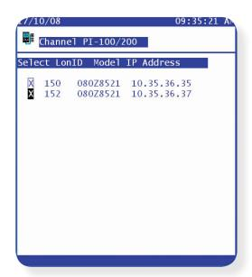
To confirm how many AKC nodes were detected navigate back to the I/O Network Status page / Overview. Select Generic to view node list. Once the correct PI gateways have been checked, perform another scan (using the Rescan Network buton). The AK-SC255 will now discover AKC nodes (max 60 per AK PI-200) attached to each PI-200
