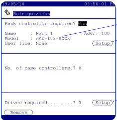
If the AKD 102 is to be used as a **pack controller**, configure AKD-102 type and use the Setup button to access drive parameters
